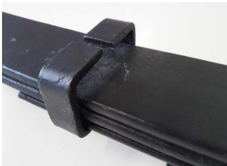
U-shaped Bracket of the leaf spring pack.
